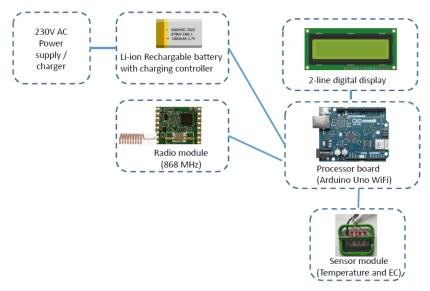
Fig. 1. Flowchart of IoT based prototype
